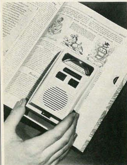
HOW THE MICROPHONOGRAPH is used. The device adds sound to the information obtainable from a printed book.
