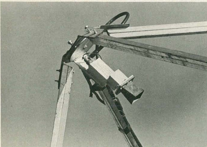
HORN ANTENNA/LNA combination points directly towards the dish antenna. Coaxial cable is used to connect the LNA to the receiver.
